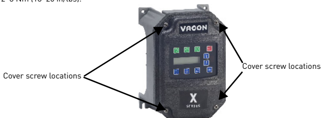
Figure 7: Vacon 50X Cover Assembly and Screw Locations
